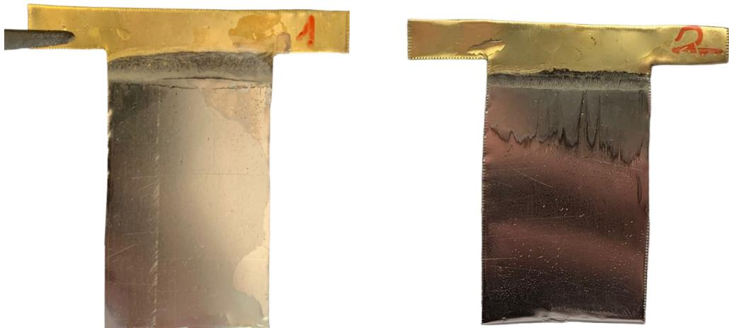
Slika 10. Uticaj zagrijavanja ( $j = 2,5 \text{ A}/\text{dm}^2$ , 50 o/min,  $T = 20^{\circ}\text{C}$ )
